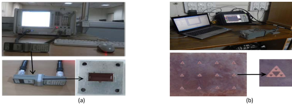
Fig. Experimental measurement setup (a) transmission-reflection waveguide setup with measured sample and, (b) ATD setup with fractal FSS embedded sample.
